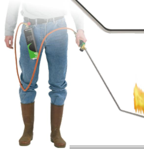
► Keep the flame at a distance of approximately 10 to 20 cm while drawing an "eight" for 2 to 4 seconds.
